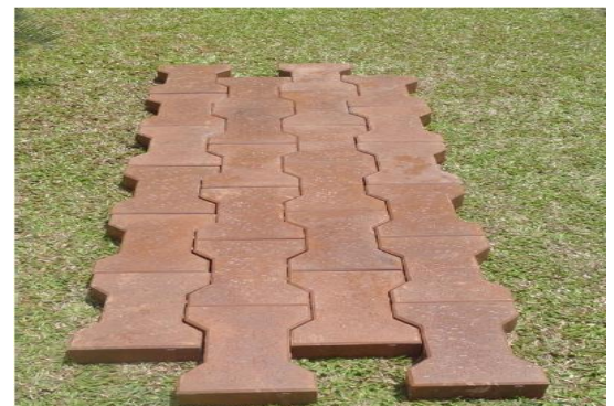
Figure 2: (a) The paver block properties obtained by Kumar and Kumar (2012); (b) The paver blocks obtained using red mud and fly
