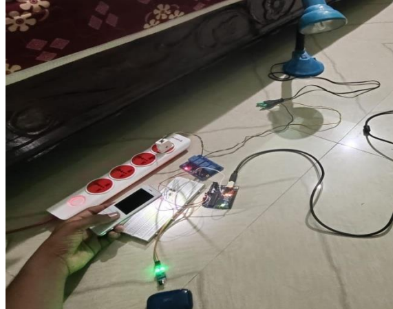
Figure10: IR detects object and light falls on LDR, light turn OFF.
